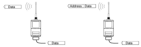
Transmission address has been set OFF. Radio modem will transmit the data packet as such. Transmission addressing has been set ON. The radio modem will add the primary TX address to the beginning of the data packet.
