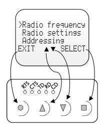
Pressing DOWN ( $\blacktriangledown$ ) button the cursor moves downwards. Depending on the sub-menu, the button also scrolls the digits of numerical values when changing some settings.
