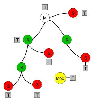
The figure left illustrates a possible structure of a radio modern network.
