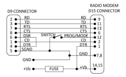
FUSE = 1 A slow ( $+6 \dots +30 \text{ V}$  assembly) or 2.5 A slow ( $+3 \dots +9 \text{ V}$  assembly) SWITCH = Programming mode switch (ON=Programming mode, OFF=Data transfer mode)
