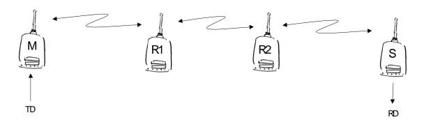
When using repeaters, the same packet is sent via a (radio) channel several times. A radio modem situated in the repeater chain will often hear other radio modems in addition to the immediate neighbouring radio modems. With Source Mode Routing the complete address information is sent
